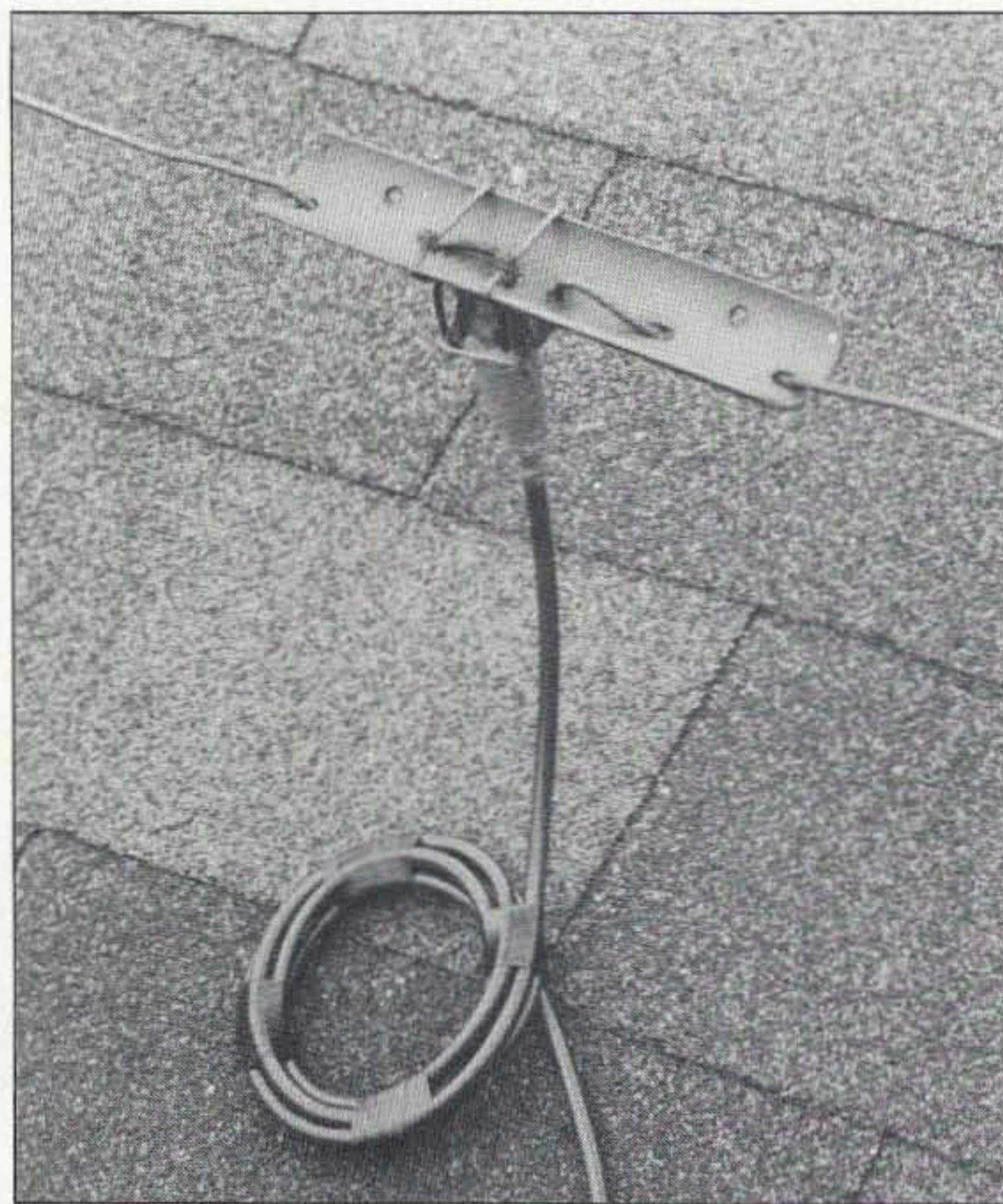
Photo C. The feed point of the baby loop antenna. A strip of PVC pipe (cut down the middle) was used to mount a SO-239 female connector and to support the antenna wire. Note also an RF air balun (1:1) formed out of coils of the feedline.
